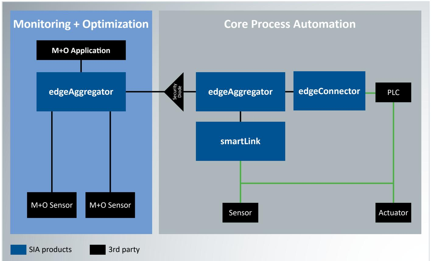
Softing Industrial offers a range of connectivity products which comply with the NOA reference architecture as outlined in the diagram above. The products provide access to machine- and process data in PLCs, as well as PLC independent access to field device data. They also support OPC UA server aggregation which can be applied on multiple levels in a complete solution, further simplifying the implementation of a second communication channel.
