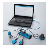
Connect the SIG200 to your computer via USB or Ethernet and start the engineering tool from SICK: SOPAS ET.
