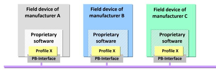
Implementation of an identical profile (X) in all devices allows consistent behavior and interoperability of the devices at the bus.
