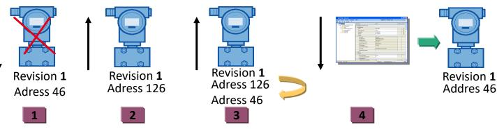
Step 1: Remove old/defect device (tagged with address 46)
