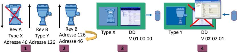
Step 1: Remove old or defect device (Rev A, Type X, tagged with address 46)
