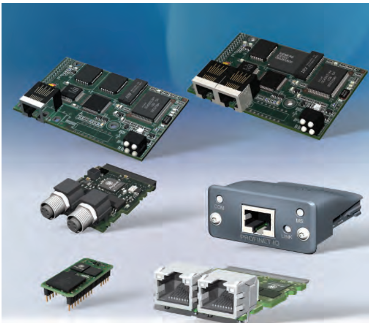
PROFINET protocol converters link field devices to PROFINET using their serial interfaces. This allows field devices to be integrated into PROFINET without any hardware or software changes to the field device.
