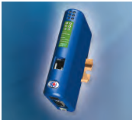
PROFINET protocol converters link field devices to PROFINET using their serial interfaces. This allows field devices to be integrated into PROFINET without any hardware or software changes to the field device.
