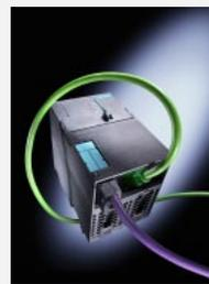
automation. PROFInet enables data interchange between intelligent devices from different manufacturers. The SIMATIC iMap tool allows communication links to be established graphically simply by drawing lines, a wonderfully user-friendly alternative to programming. **Siemens: [www.siemens.de/cba](http://www.siemens.de/cba).**
