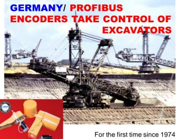
One of the largest German open cast lignite mining areas is situated in the Rhineland to the west of Cologne. There, huge bucketwheel excavators are employed by the Rheinbraun company, measuring up to 240 meters in length and almost 100 meters in height. They have a capacity of 240.000 m³ per day.
