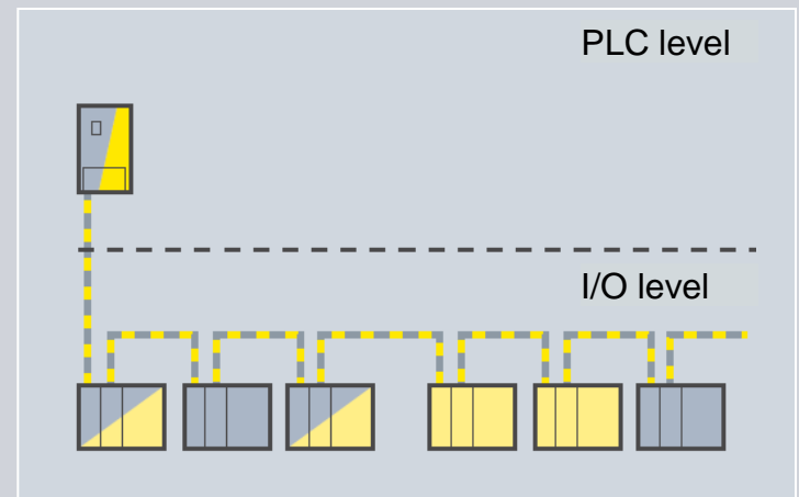
One PLC, one bus and mixed I/O
